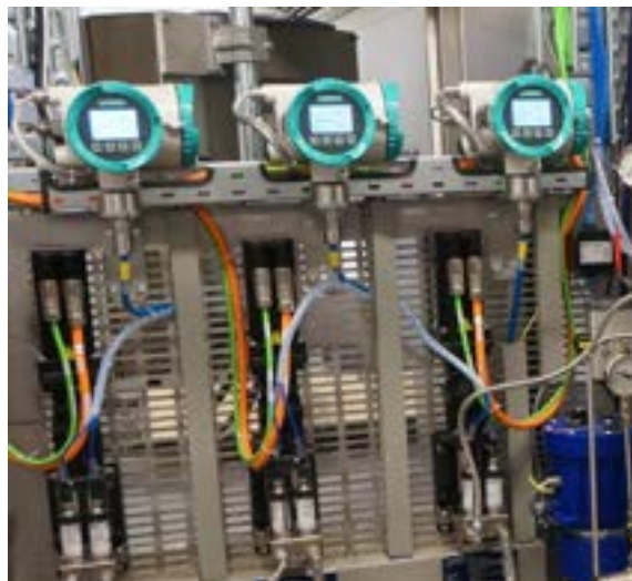
dosing by gear pumps, measuring by coriolis system
